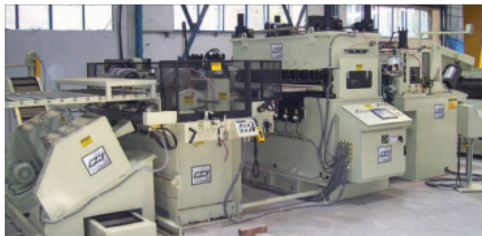
CTL System features a B&K precision corrective leveler
