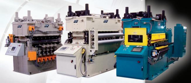
Available in standard 4-high and optional 5- or 6-high roll arrangements with material width capacities from 18" to 96". Ensure dead-flat panel or strip for increased productivity and part quality with B&K levelers.
