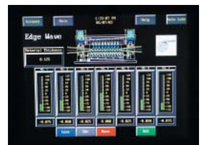
Preset back up roll adjustments based on edge wave condition
